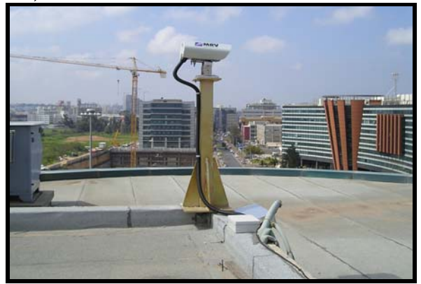
Figure 2.7: Floor Pedestal Mounting (using JMP and M015C)
